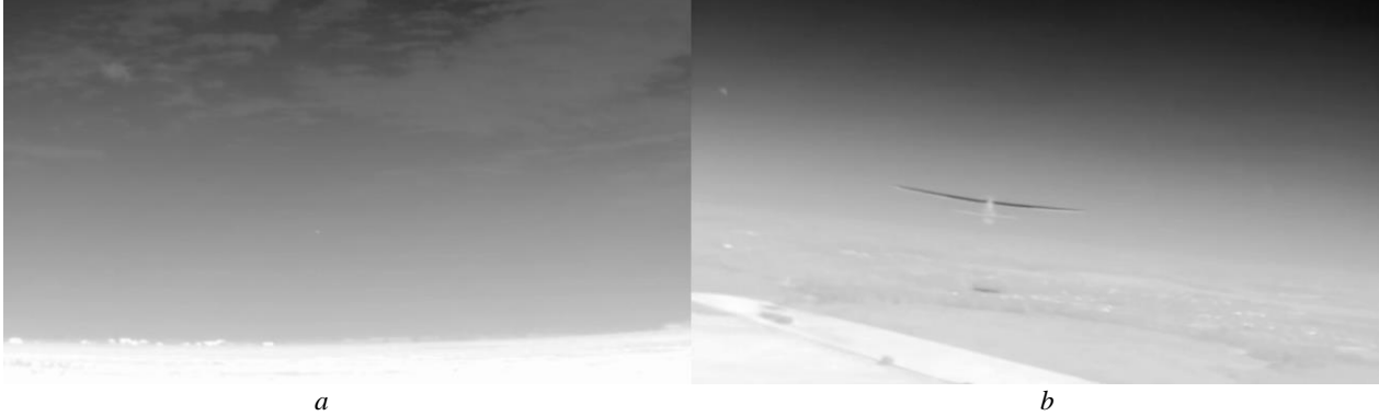
FIG. 1. Real thermal seed images used for video diffusion: a – Seed A – far-field IRSTD-scale fixed-wing UAV at 700 m range, appearing as a blurry thermal dot; b – Seed B – near-field fixed-wing UAV at <50 m, with a resolved airframe and clearly visible hot engine region. These two seeds anchor the multiscale dot-to-object continuum modeled in Gen-Thermal-UAV
